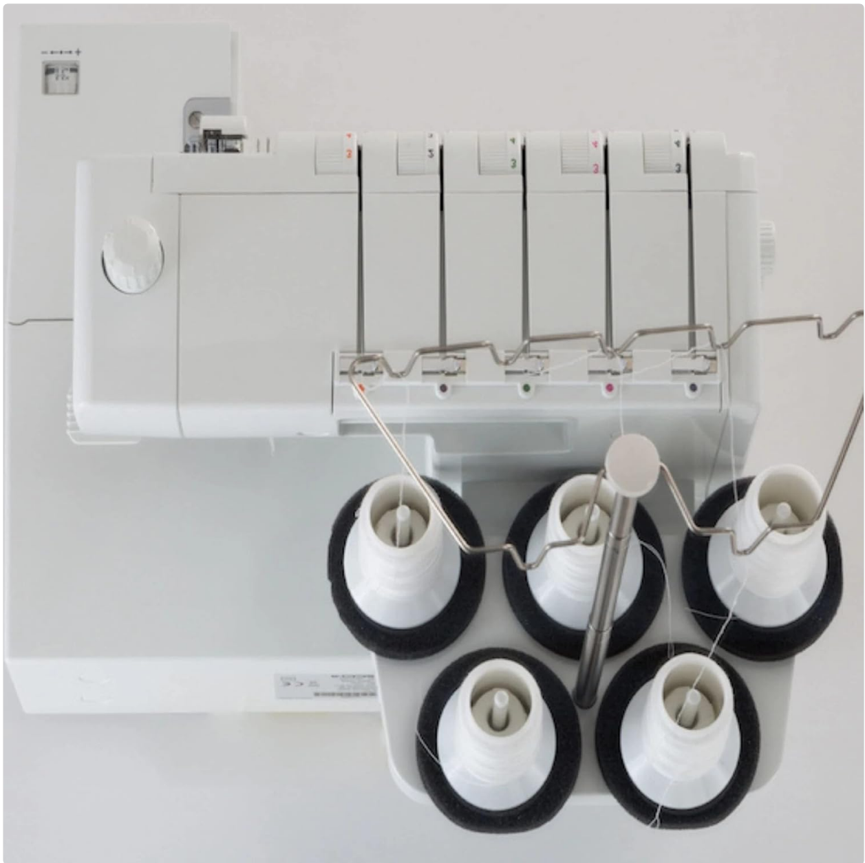
Figure 1: Top view of the Necchi NCV10A machine, illustrating the placement of thread spools on the spool pins and the initial path through the thread guides. This view is crucial for understanding the threading process.
