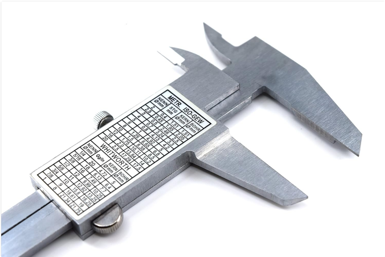
Image 4.1: The reverse side of the caliper features useful conversion tables.
