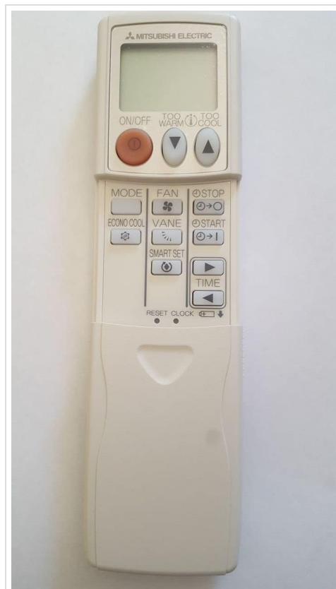
Figure 1: Front view of the E1209C426 Remote Controller. This image displays the remote's layout, including the LCD screen at the top, followed by the main power button, temperature adjustment buttons, and various function buttons such as MODE, FAN, VANE,
