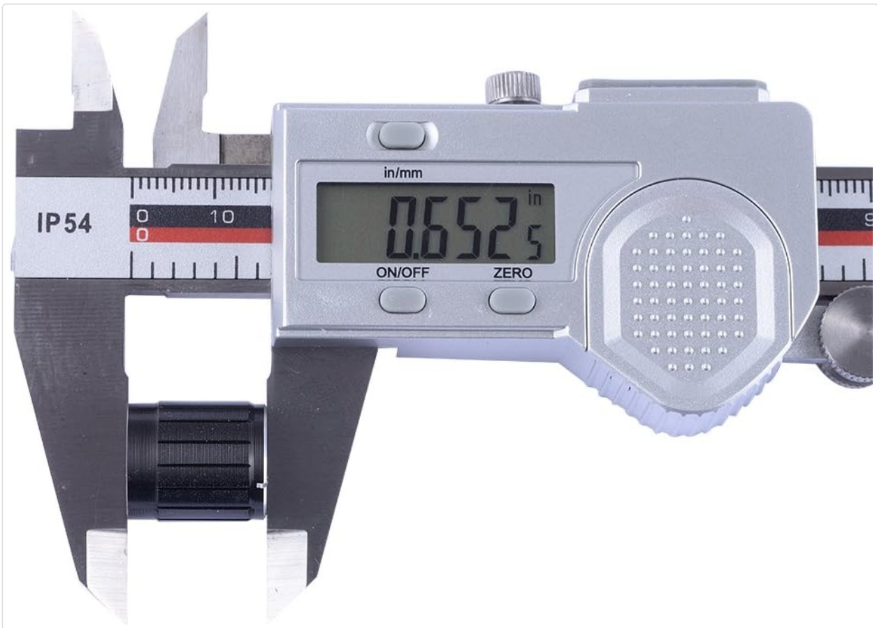
Figure 6: A digital caliper measuring the height of a knob cap, showing a reading of approximately 0.652 inches.
