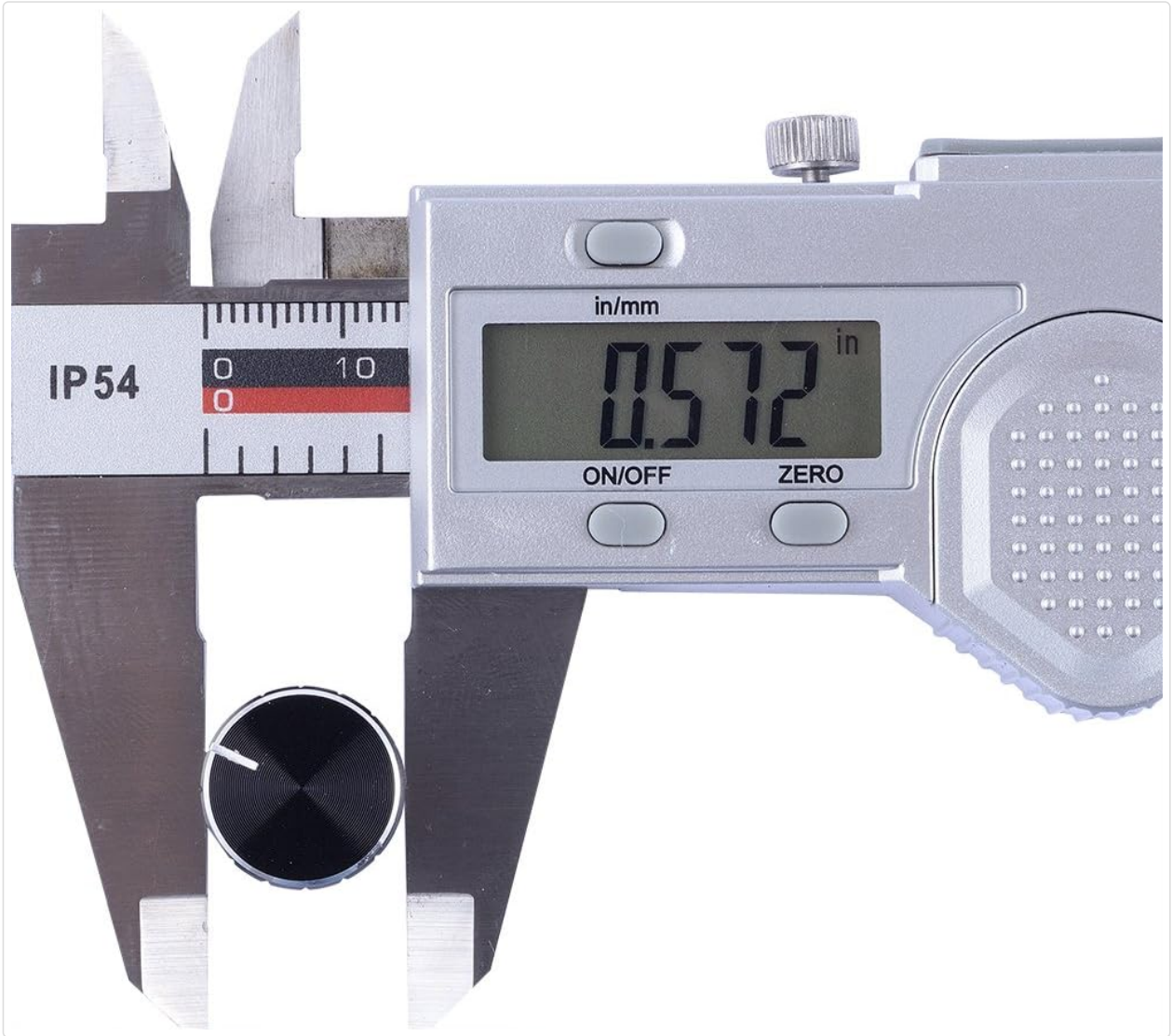
Figure 5: A digital caliper measuring the diameter of a knob cap, showing a reading of approximately 0.572 inches.
