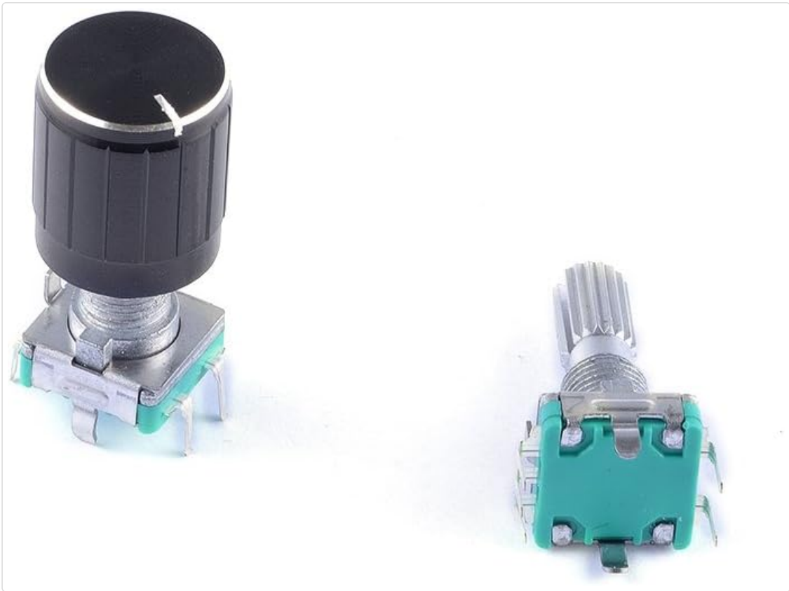
Figure 4: An assembled Cylewet CYT1100 rotary encoder with its knob cap, alongside a separate encoder unit without the cap.
