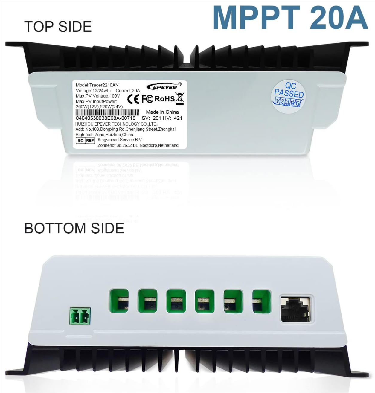
Image 3.2: Top and bottom views of the EPEVER Tracer2210AN controller. The top view shows the model information and certifications, while the bottom view displays the terminal connections and communication port.
