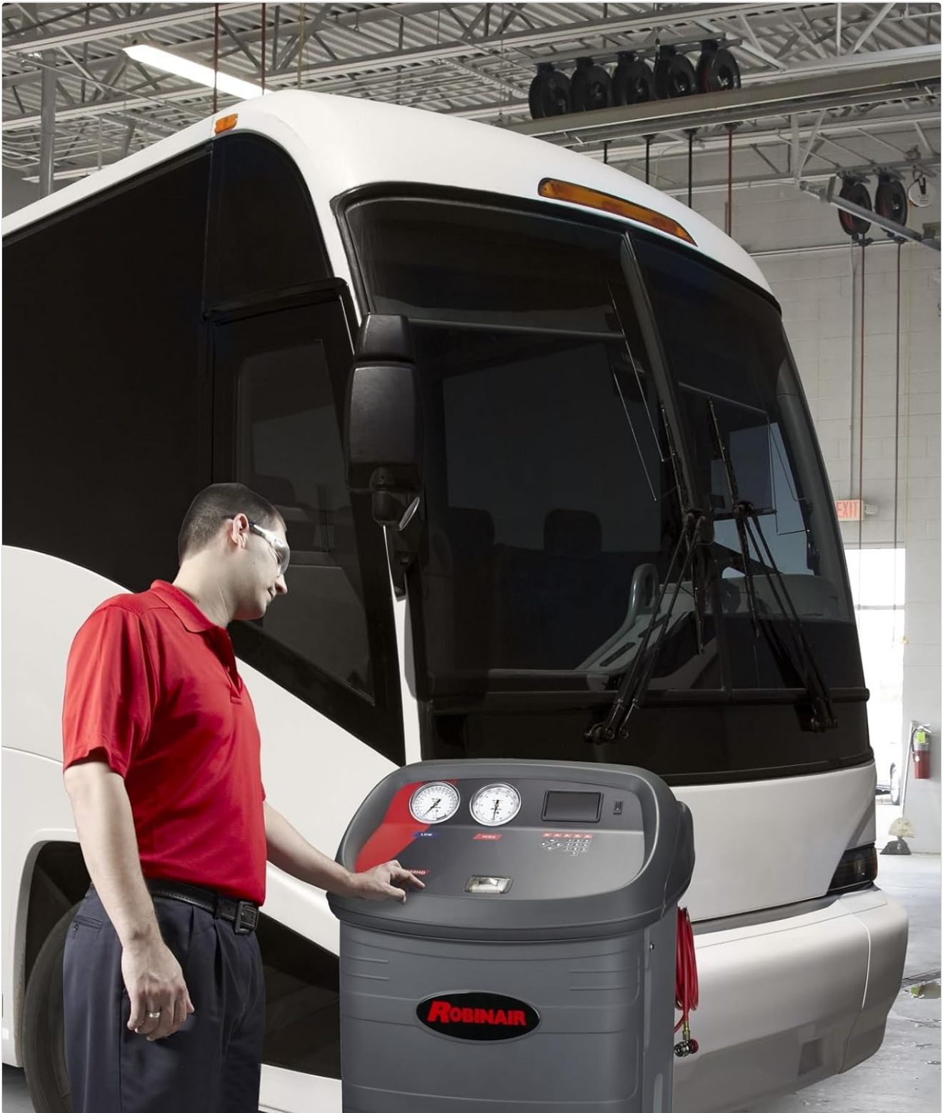
Figure 2: A technician operating the Robinair 34888HD machine next to a large bus, demonstrating its heavy-duty application for oversized vehicles.
