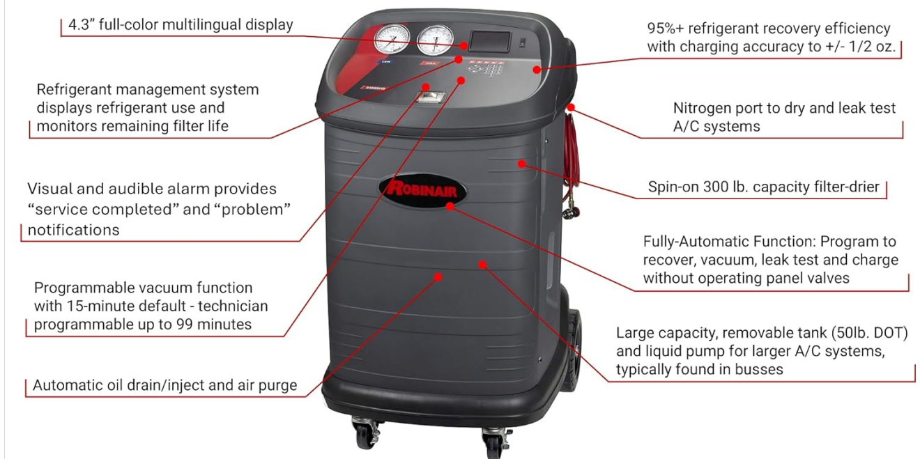
Figure 1: Detailed diagram highlighting the key features of the Robinair 34888HD machine, including the 4.3" full-color multilingual display, refrigerant management system, nitrogen port, spin-on filter-drier, fully-automatic function, programmable vacuum, automatic oil drain/air purge, and large capacity removable tank.
