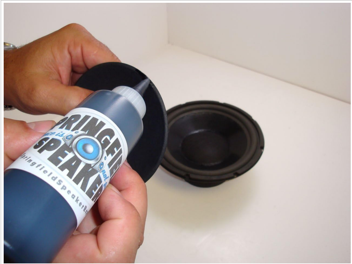
Image 4.1: A hand applying the black rubberized adhesive to the edge of a speaker cone, preparing it for surround attachment.
