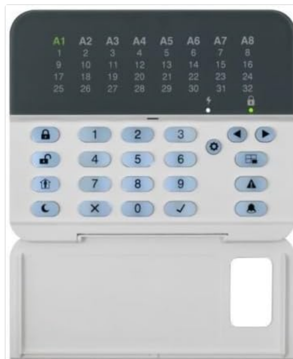
Figure 3.2: Telettek LED 32 Keypad with open cover, revealing the full numeric and function button layout. Below the LED display, a full set of numeric keys (0-9), navigation arrows, and dedicated function buttons for arming, memory, troubles, and bypassed zones are visible.
