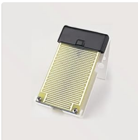
Figure 8: Leaf Wetness Sensor. This sensor detects moisture on plant surfaces, aiding in disease prevention.
