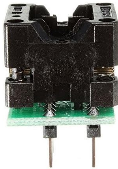
Figure 3.1: Close-up of the SOP8 socket, showing the mechanism for securing the IC.
