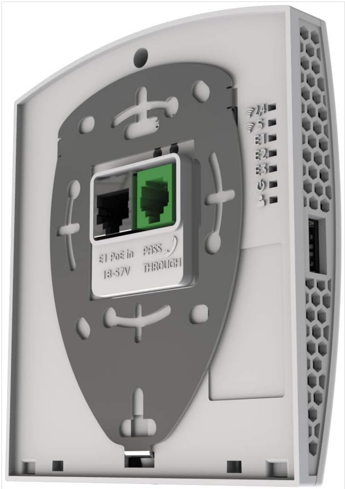
Figure 2: Detailed view of the rear panel of the MikroTik wsAP ac lite. This image highlights the E1 PoE-in Ethernet port, E2 and E3 LAN ports, USB 2.0 port, and the RJ11 pass-through telephone jack, along with mounting plate attachment points.
