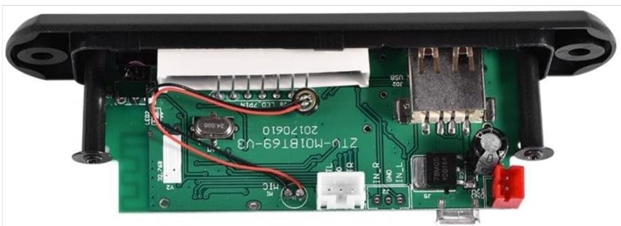
Figure 3.1: Rear view of the decoder board, illustrating the wiring points for power and audio output.
