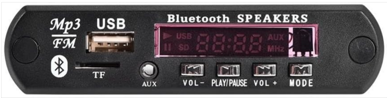
Figure 2.1: Front view of the decoder board, highlighting the USB port, TF card slot, display, and control buttons.
