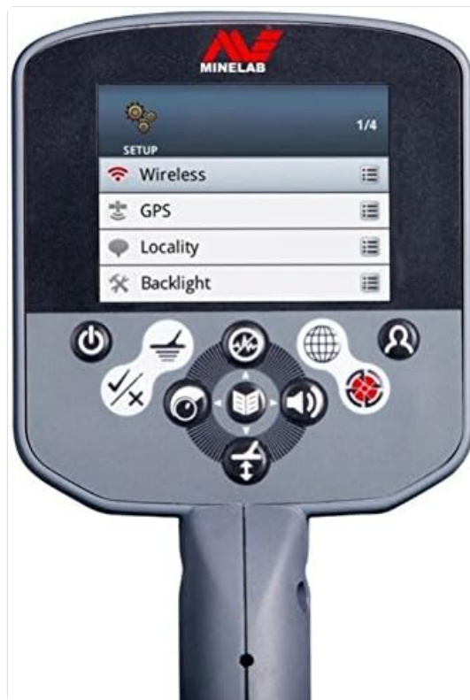
Figure 3.2: Close-up view of the CTX 3030's full-color LCD control panel, displaying various settings and navigation buttons for operation.
