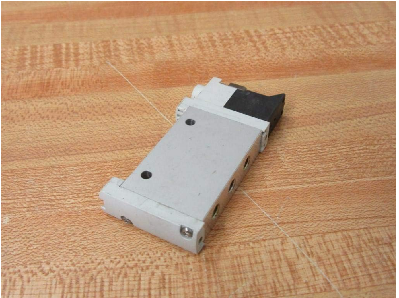
Figure 4.2: Bottom view of the valve, illustrating the M5 pneumatic working ports.
