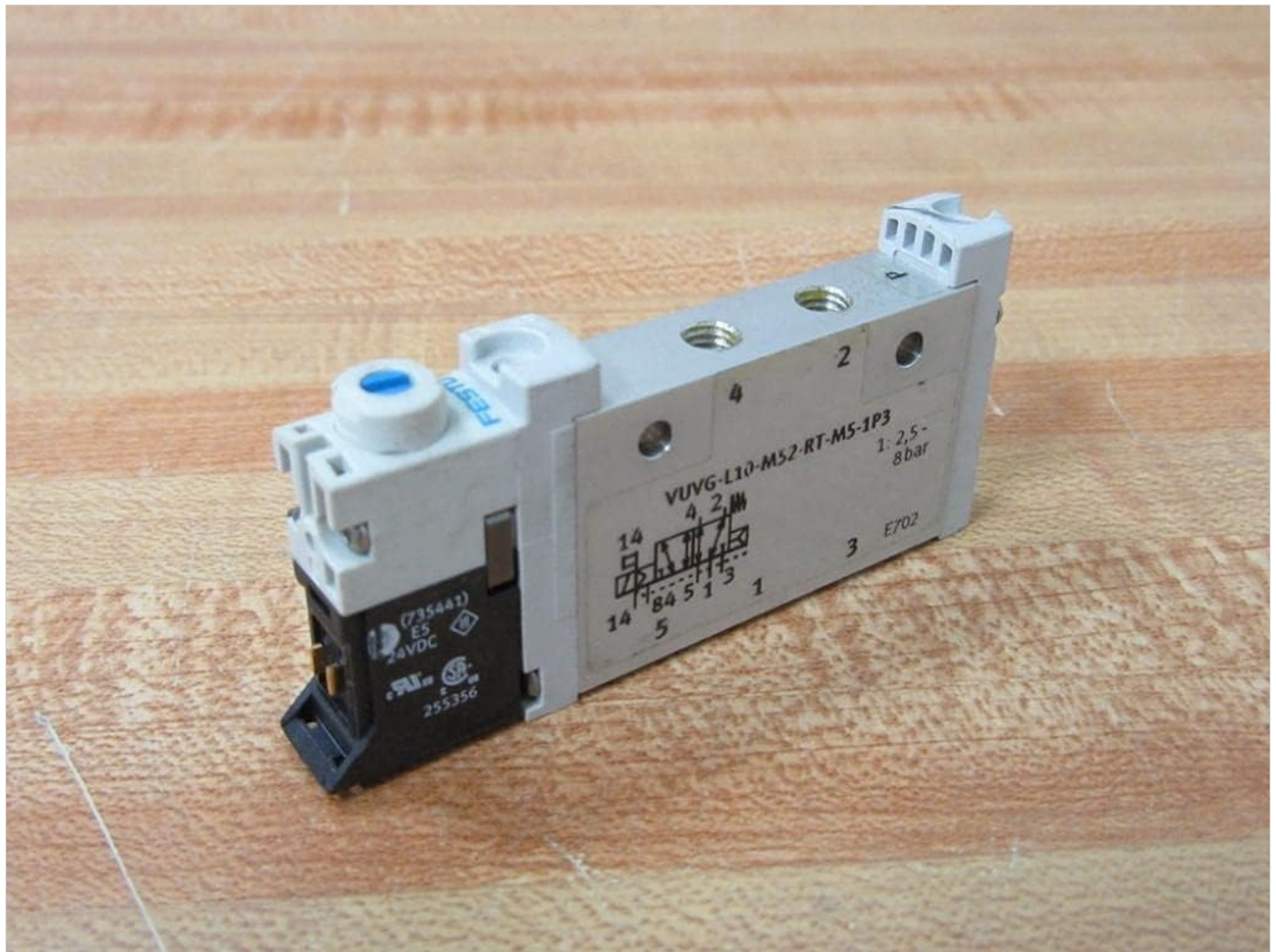
Figure 3.1: Overall view of the FESTO VUVG-L10-M52-RT-M5-1P3 air solenoid valve.
