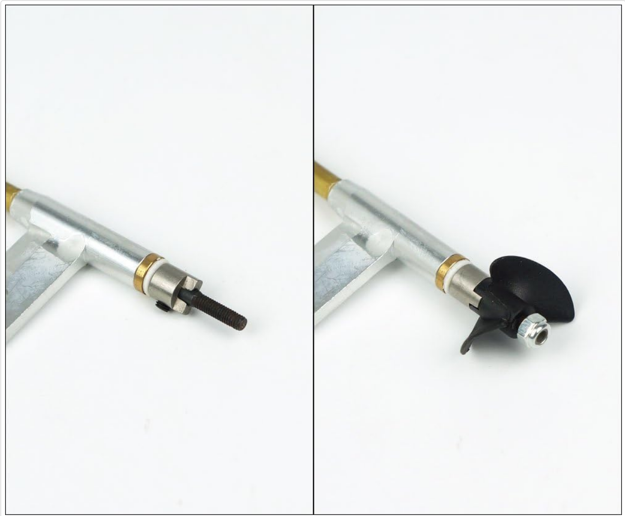
Image: The propeller shaft assembly, showing the shaft before and after the propeller is securely attached.
