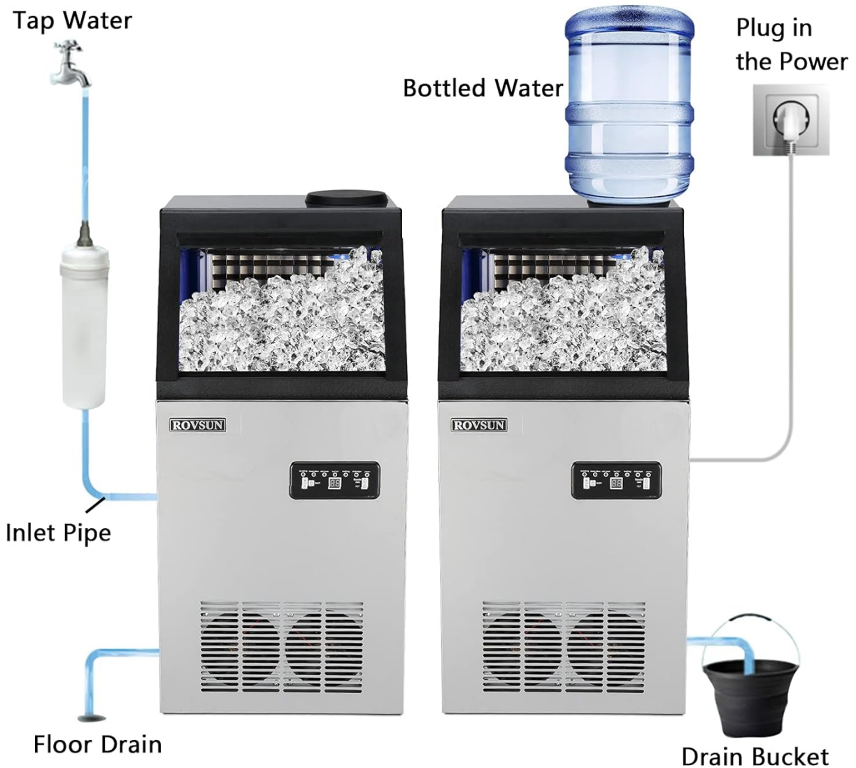
Figure 3: Illustration of connecting the ice maker to either a tap water supply with a filter and floor drain, or using bottled water with a drain bucket.
