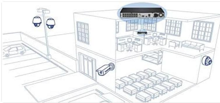
This diagram illustrates a typical deployment scenario for the TRENDnet TV-NVR416 NVR system, showing how the NVR integrates with various camera types in different environments, such as indoor offices and outdoor areas, to provide comprehensive surveillance coverage.
