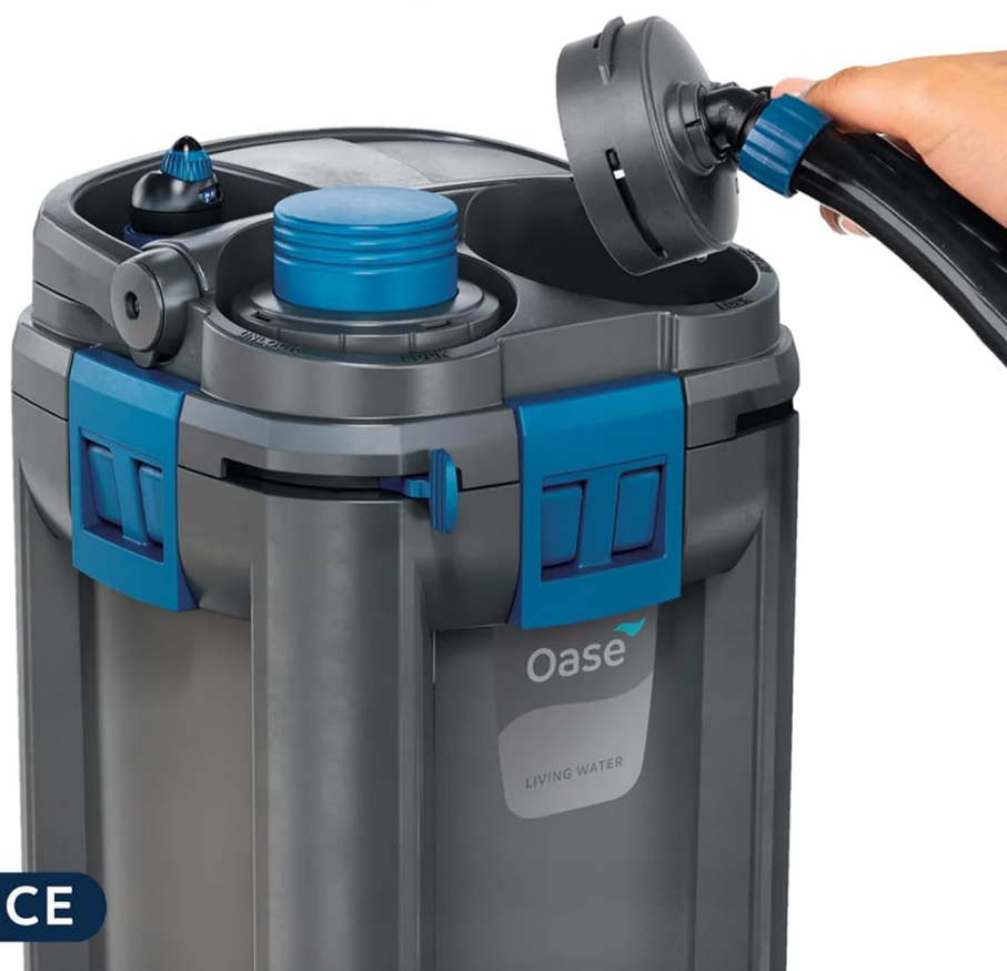
Figure 6.2: The aquastop feature on the OASE BioMaster filter, allowing for easy disconnection of hoses from the filter head without water spillage during maintenance.
