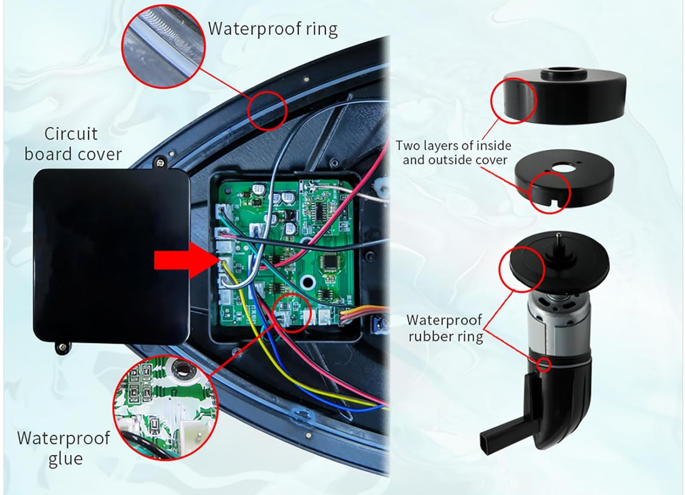
Figure 5: Detailed view of the boat's enhanced waterproofing features, including the waterproof ring, circuit board cover, and waterproof rubber ring, ensuring suitability for various water conditions.
