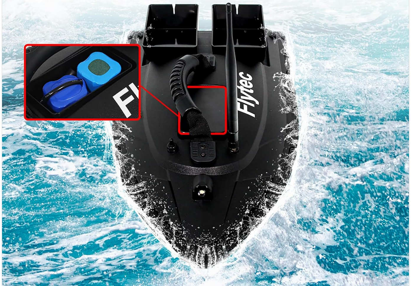
Figure 1: The battery compartment is designed to accommodate two battery sets for extended operation. Ensure the compartment is
