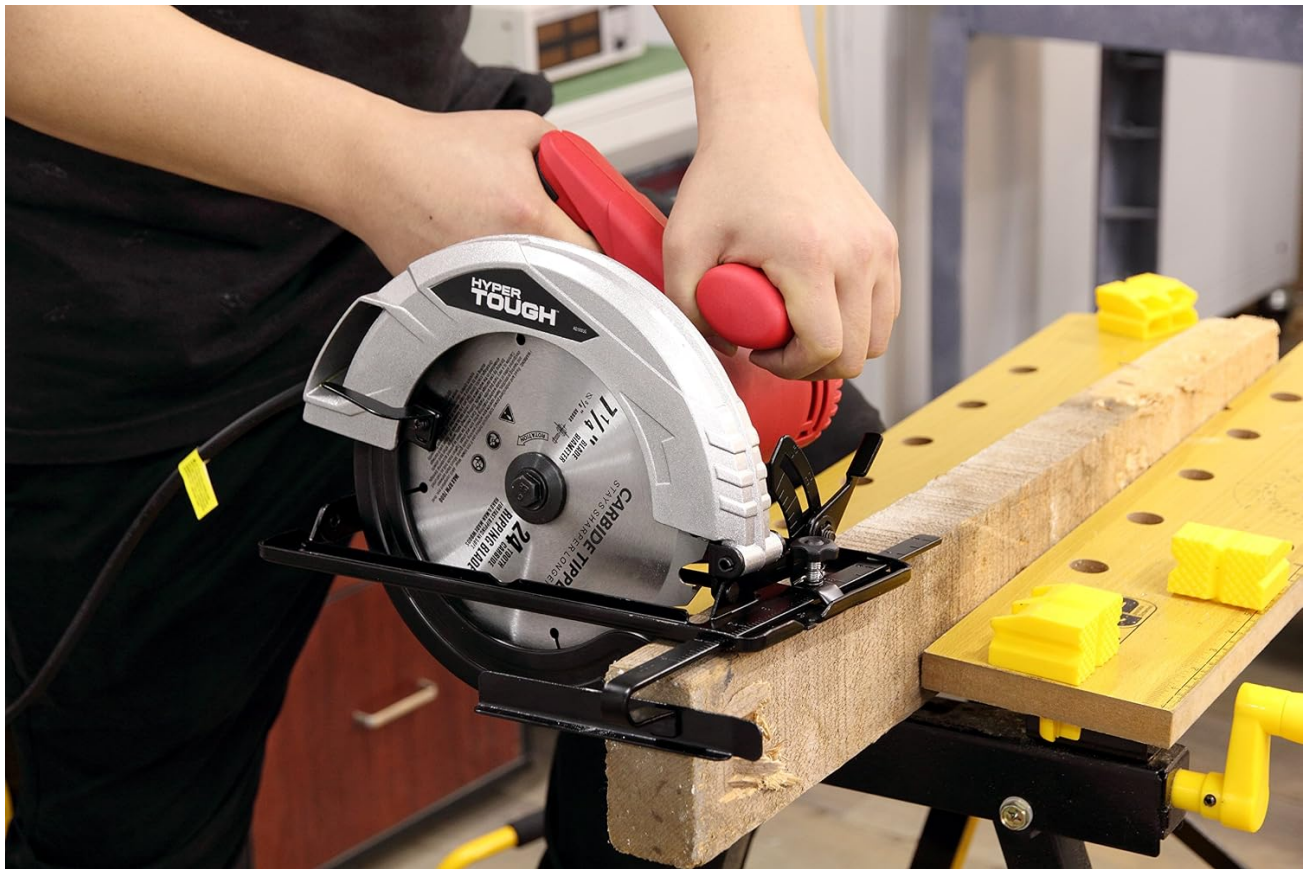
Figure 5.1: A user demonstrating the proper technique for operating the Hyper Tough circular saw to make a straight cut on a wooden board, emphasizing secure workpiece placement.
