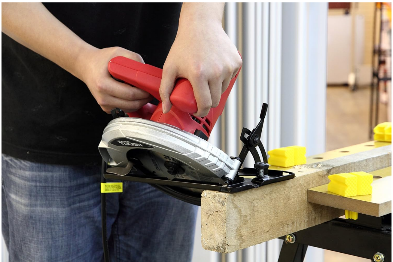
Figure 4.1: Demonstrating the adjustment of the bevel angle on the circular saw, allowing for angled cuts up to 45 degrees.
