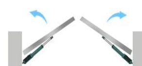
Gate Swing Out Push-to-open Installation Mode
