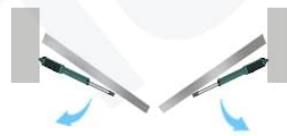
Gate Swing In Pull-to-open Installation Mode
