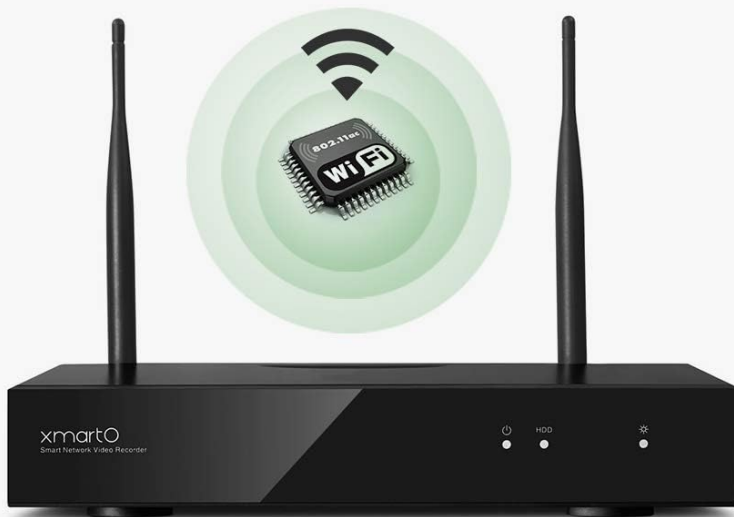
Image 3.3: Illustration of the xmartO NVR's built-in router, which creates a dedicated wireless network for the cameras, reducing reliance on home Wi-Fi.
