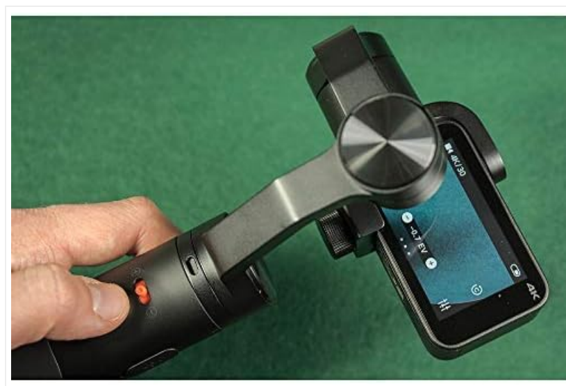
Figure 4: Proper mounting of the Mi Action Camera onto the stabilizer's cradle.
