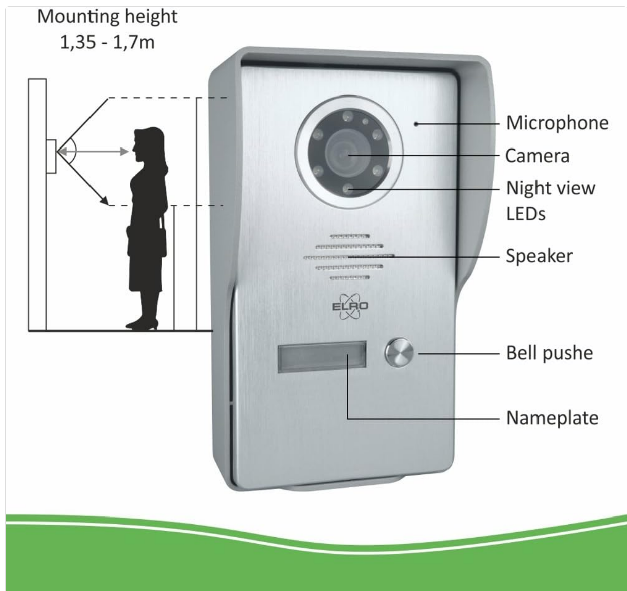
Image 2.1: Diagram illustrating the components of the outdoor unit, including the microphone, camera, night view LEDs, speaker, bell push button, and nameplate.
