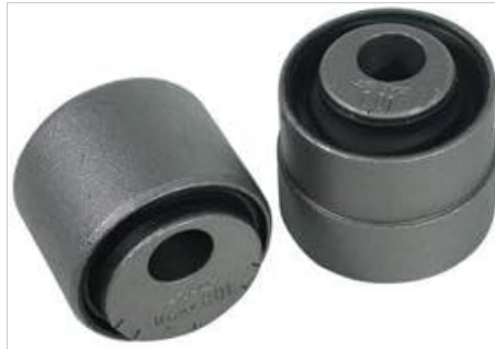
Figure 2: A pair of SPC Control Arm (66050) bushings. These components are designed to fit precisely into the control arm, providing a secure pivot point and reducing unwanted movement in the suspension.
