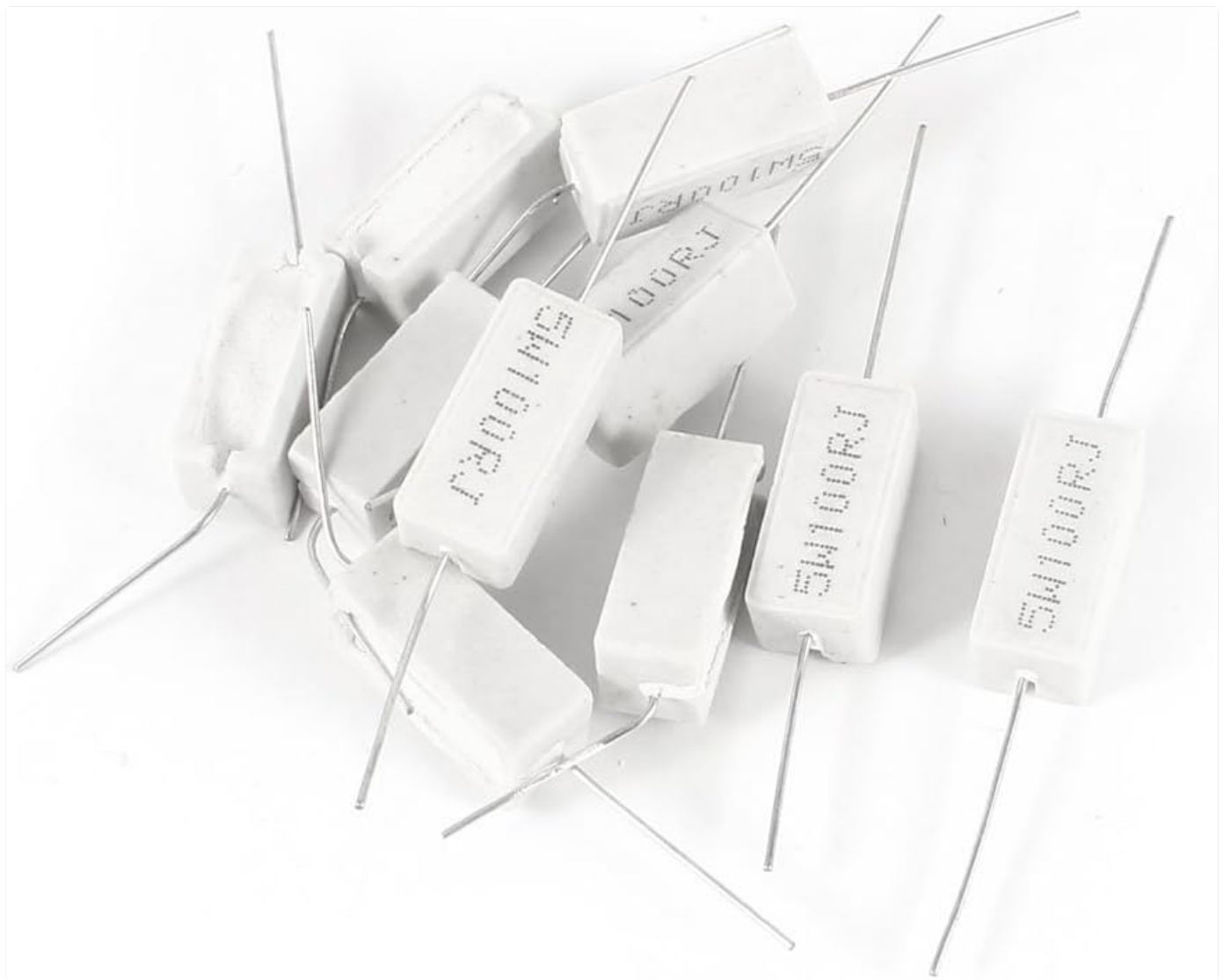
Figure 1: A group of Aexit 5W 100 Ohm ceramic cement resistors. Each resistor is rectangular, white, and features two metal axial leads extending from its ends. The resistance value '5W100RJ' is printed on the body of some resistors, indicating 5 Watts and 100 Ohms with a 5% tolerance.
