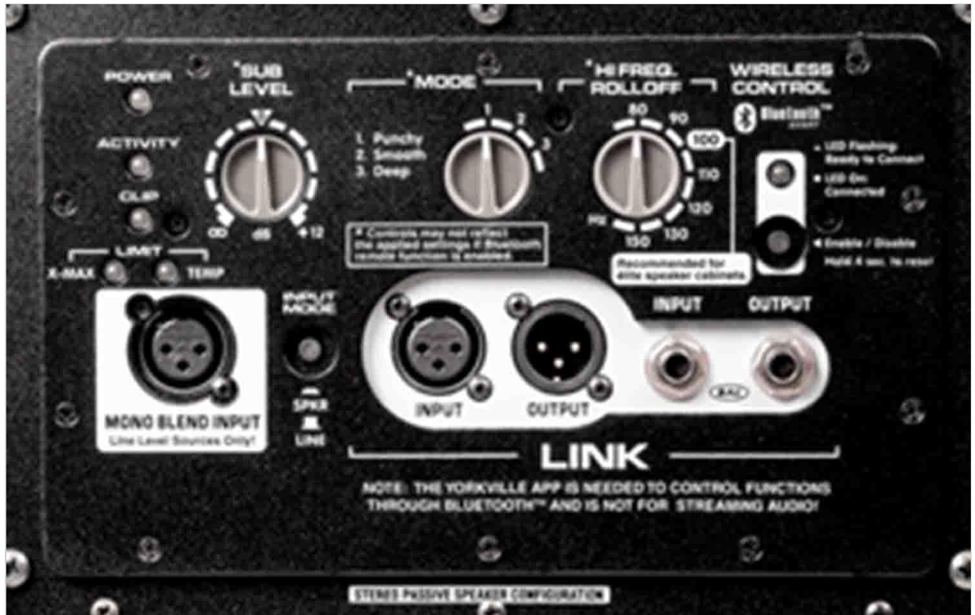
Figure 4: Detailed view of the control panel, including SUB LEVEL, MODE, HI FREQ ROLLOFF, and Wireless Control sections.
