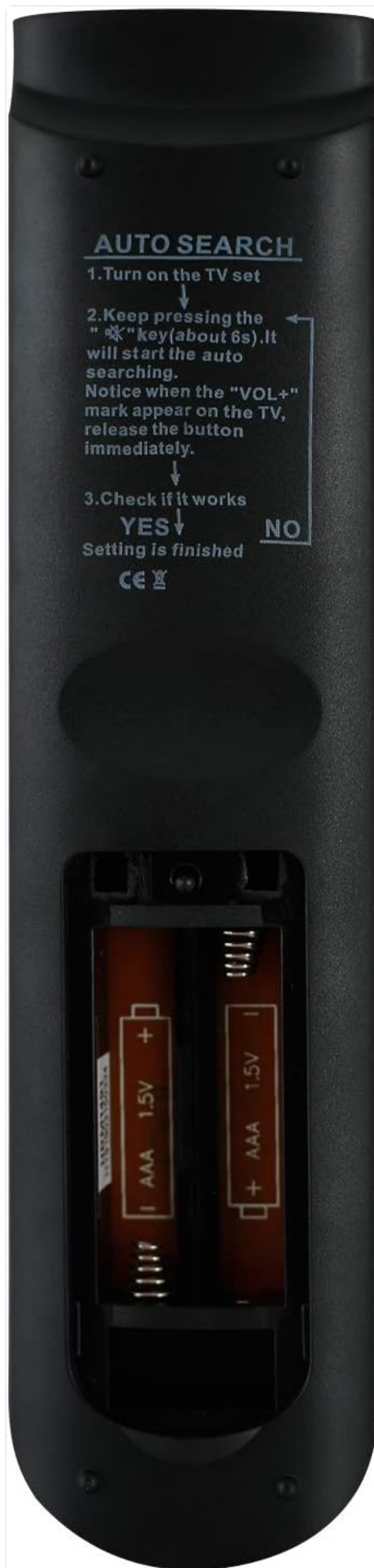
Image: Back view of the remote control with the battery compartment open, showing the slots for two AAA batteries with polarity markings.
