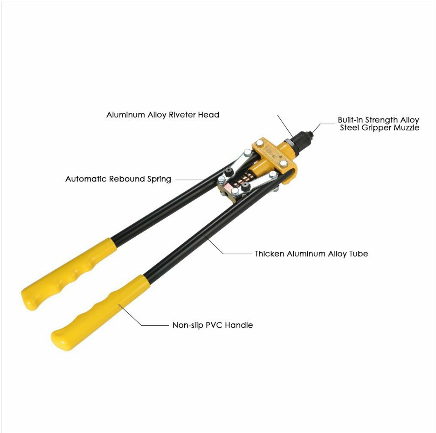
Figure 2: Key components of the rivet gun. Features include an aluminum alloy riveter head, a built-in strength alloy steel gripper muzzle, an automatic rebound spring, a thickened aluminum alloy tube, and non-slip PVC handles for comfortable and secure grip.
