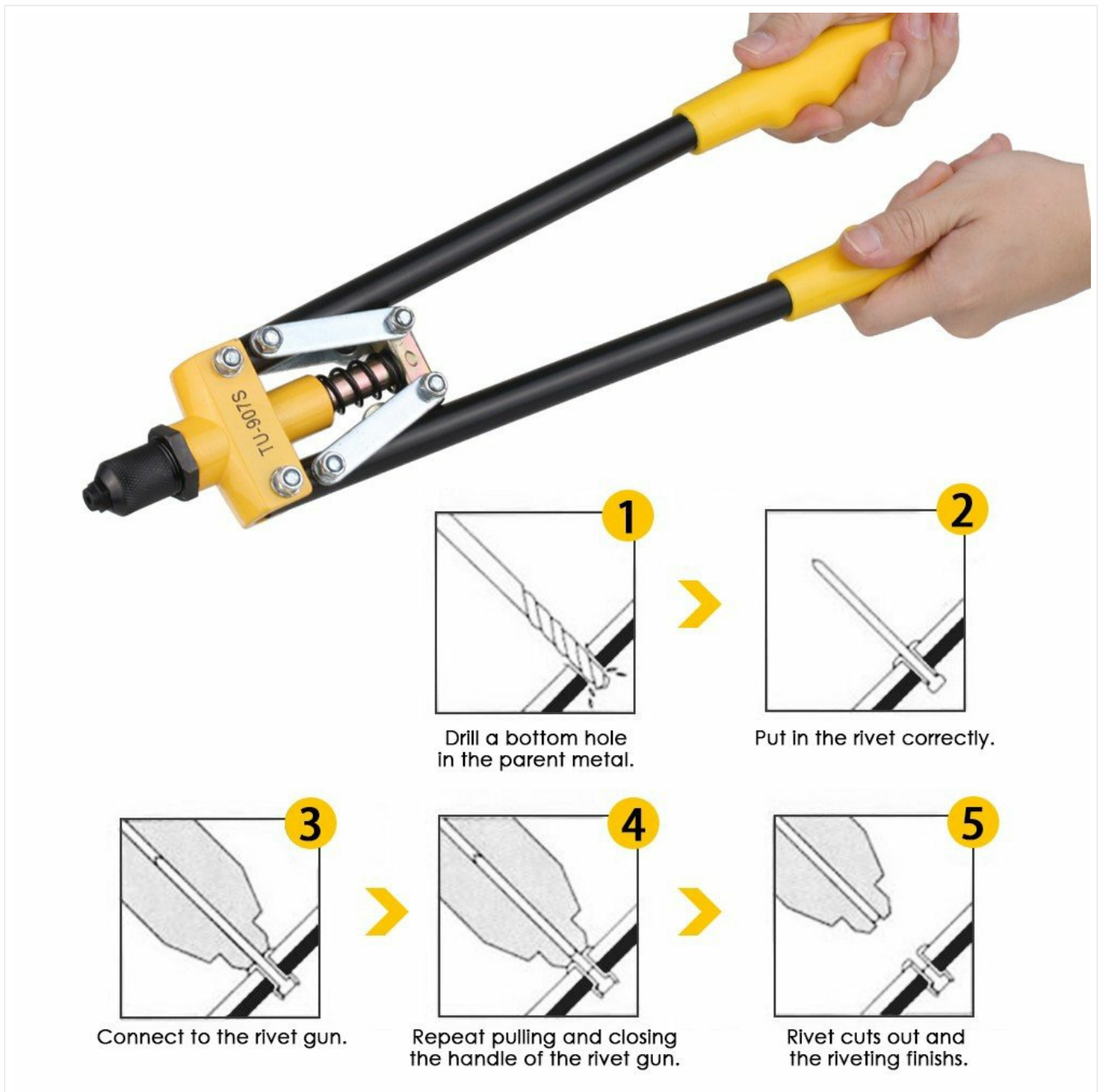
Figure 4: Visual guide for the riveting process.
