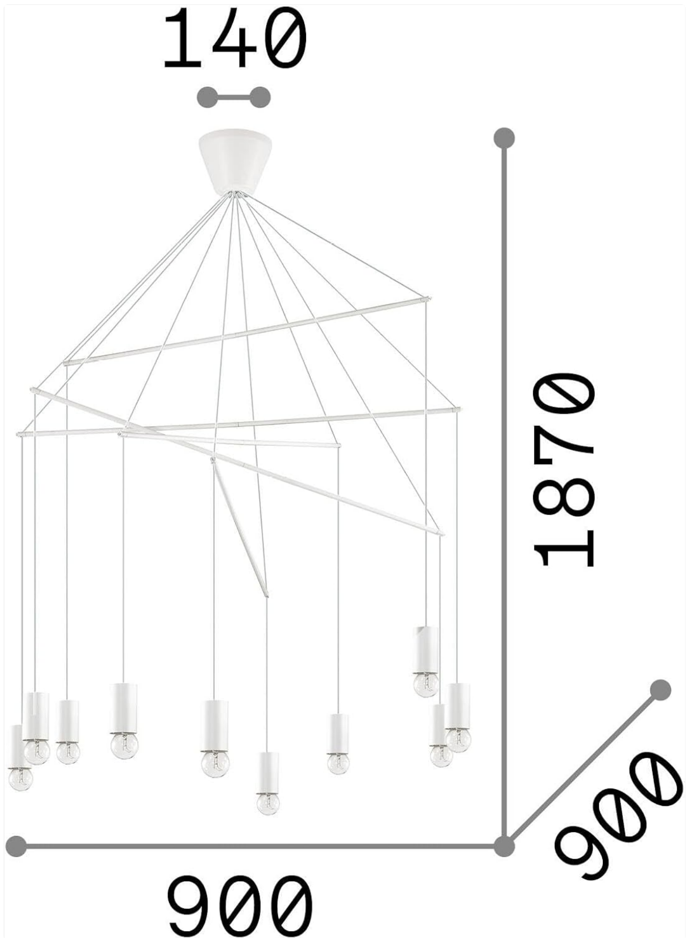
Figure 2: Dimensional Diagram of the POP SP10 NERO. This diagram illustrates the key measurements of the lamp, including its maximum height, width, and the diameter of the ceiling rose.
