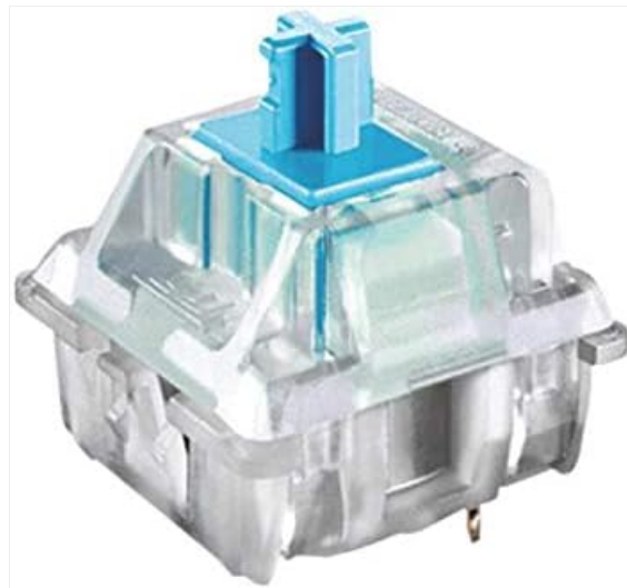
Image 5.1: Close-up of a Cooler Master Blue Mechanical Switch.
