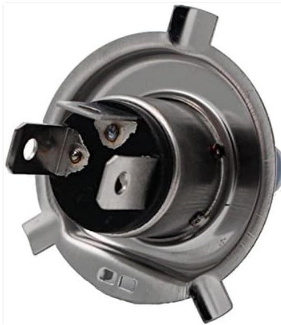
Image 3.2: The rear view of an OSRAM H4 headlight bulb, showing the three electrical terminals on its base.
