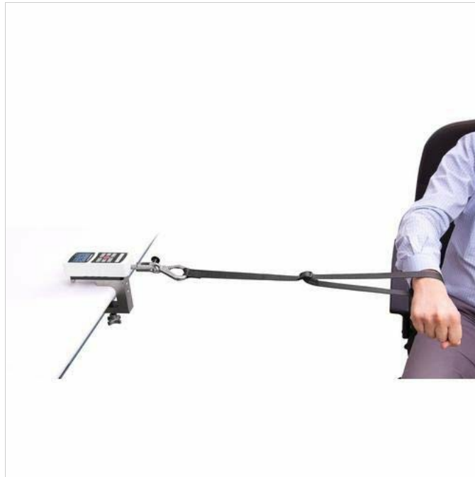
Figure 2: Example setup of the EKM5-200 Myometer Kit for an ergonomics study, showing the force gauge mounted on a table and connected to a subject via a strap.
