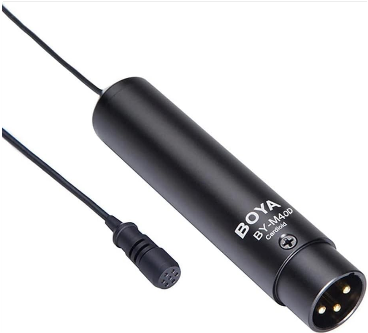
Image 2: Detailed view of the BOYA BY-M4OD main unit, displaying the brand name and model number, with the small lavalier microphone head connected via its thin cable.
