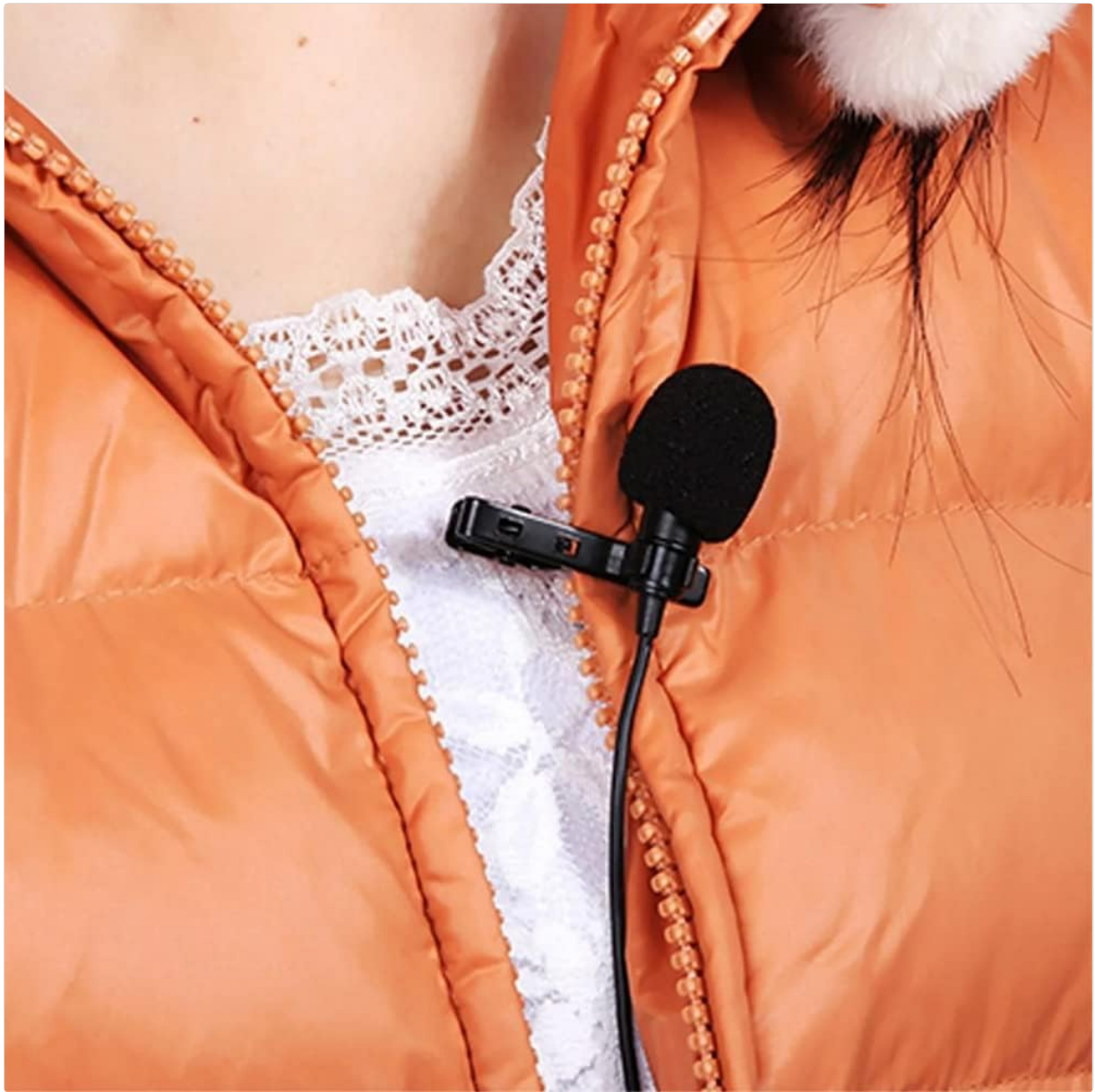
Image 3: Example of the lavalier microphone correctly clipped onto a jacket, demonstrating typical placement for recording.
