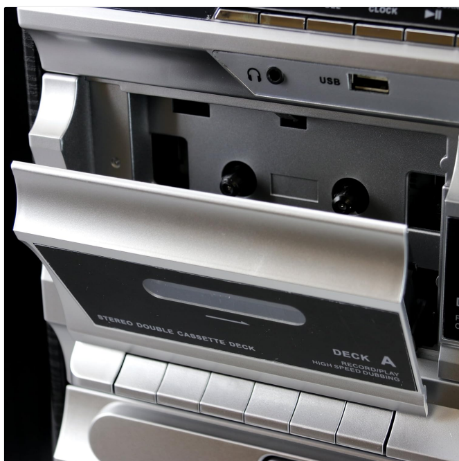
Figure 4: A detailed view of Cassette Deck A, showing the open cassette door and control buttons below.
