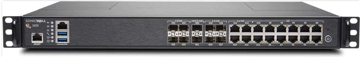
Figure 4.1: Front view of the Sonicwall NSA 3650 appliance, showing the Sonicwall logo, model number, status LEDs, management ports (MGMT, Console/DBG), USB ports, and various Ethernet ports (1GE, 2.5GE, 10GE) with corresponding port numbers (X1-X24).
