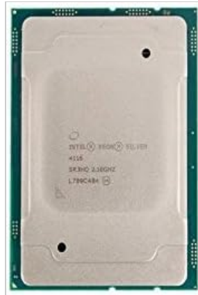
Image: Top view of the Intel Xeon Silver 4116 processor, showing the integrated heat spreader and Intel branding.
