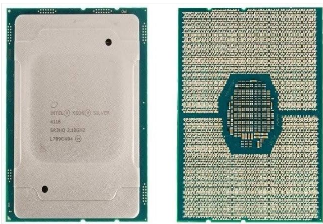
Image: Side-by-side view of the Intel Xeon Silver 4116 processor, displaying both the top (integrated heat spreader) and bottom (LGA 3647 contact array) surfaces.
