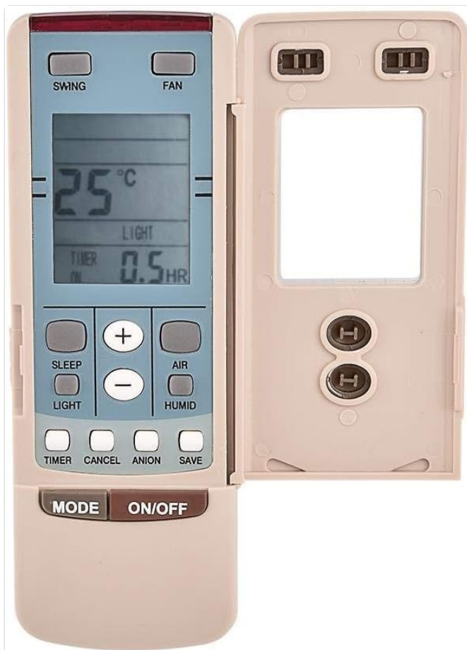
Figure 3: Remote control with sliding cover open, showing advanced function buttons.
