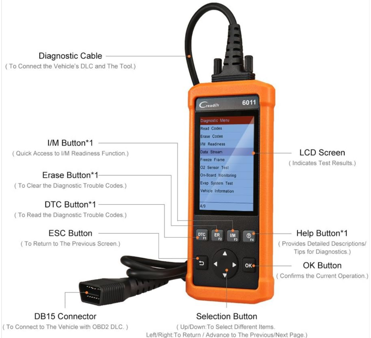
Figure 5.1: Key components and button functions of the Creader 6011.
