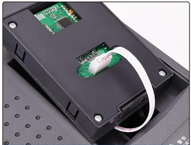
② 4 pins 20cm connection cable 4 pins cable for Digital panel
