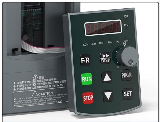
④ Removable Digital panel Digital panel can removable,bring convenience operation for numerical control machine, we can add Extension cord for you,pls contact the customer service for the price.
