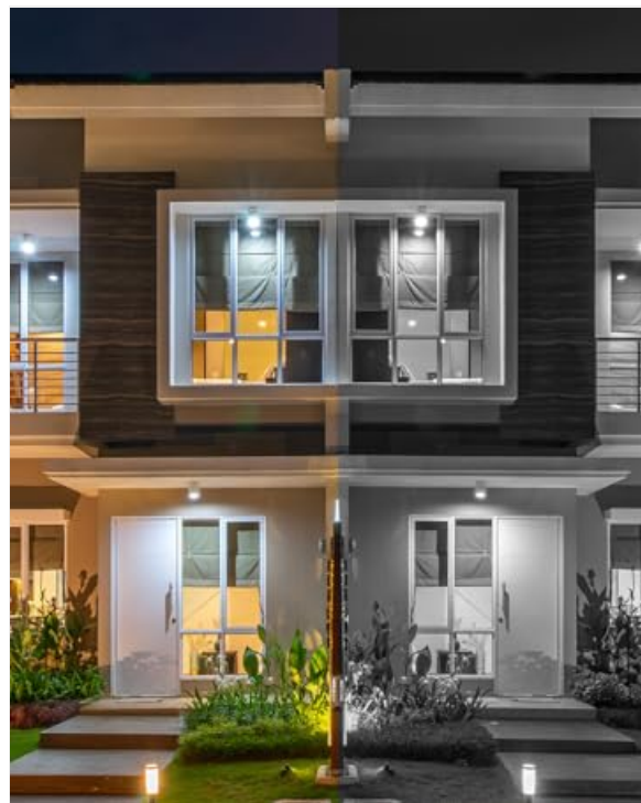
Figure 4.1: Demonstration of enhanced color night vision using spotlights and IR LEDs.
