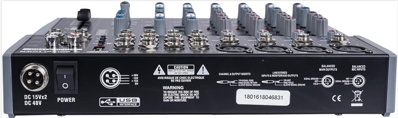
Image: The rear panel of the Sound Town TRITON-A12BD mixer, displaying the power input (DC 15Vx2, DC 48V), USB interface port, balanced main outputs, and balanced mic inputs.
