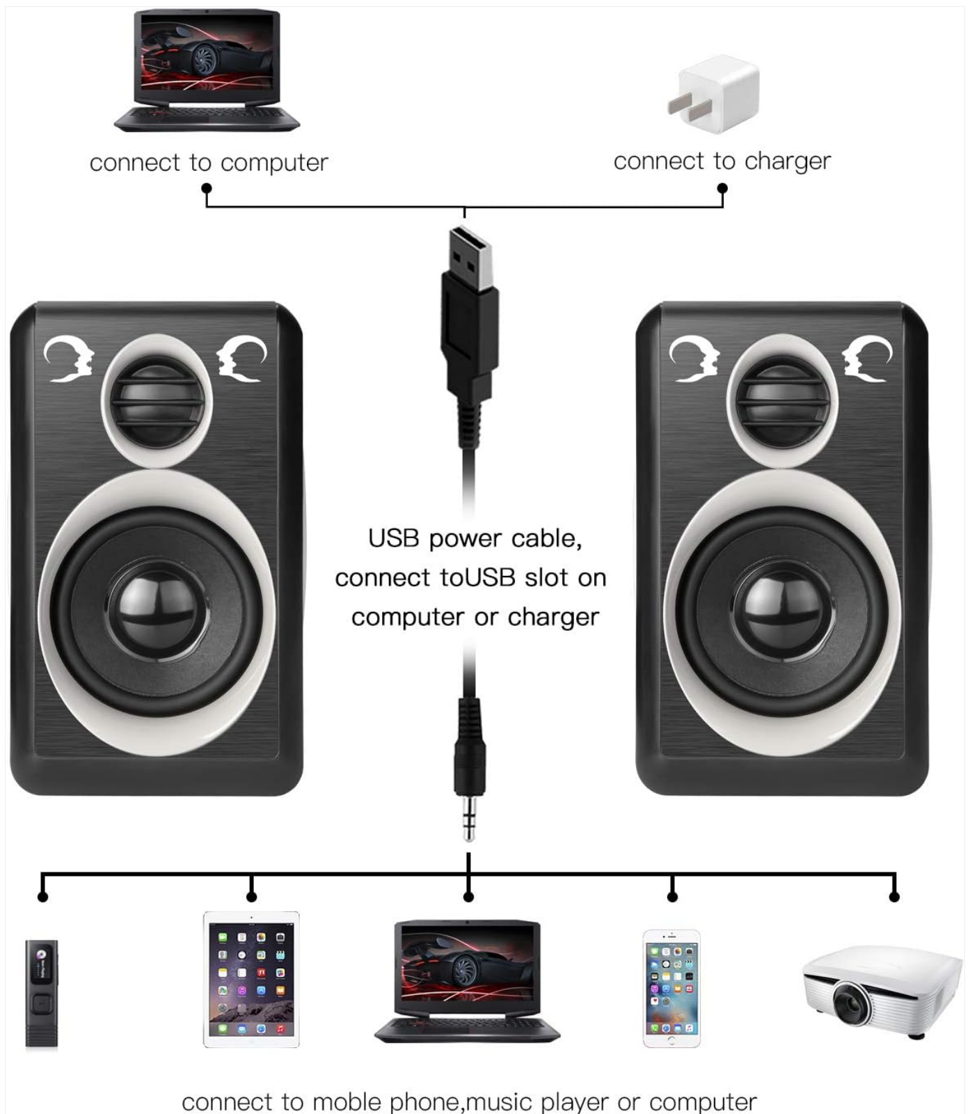
Image: Diagram showing how to connect the RECCAZR MP2000 speakers to various devices like mobile phones, music players, laptops, and projectors, using the USB power cable and 3.5mm audio jack.
