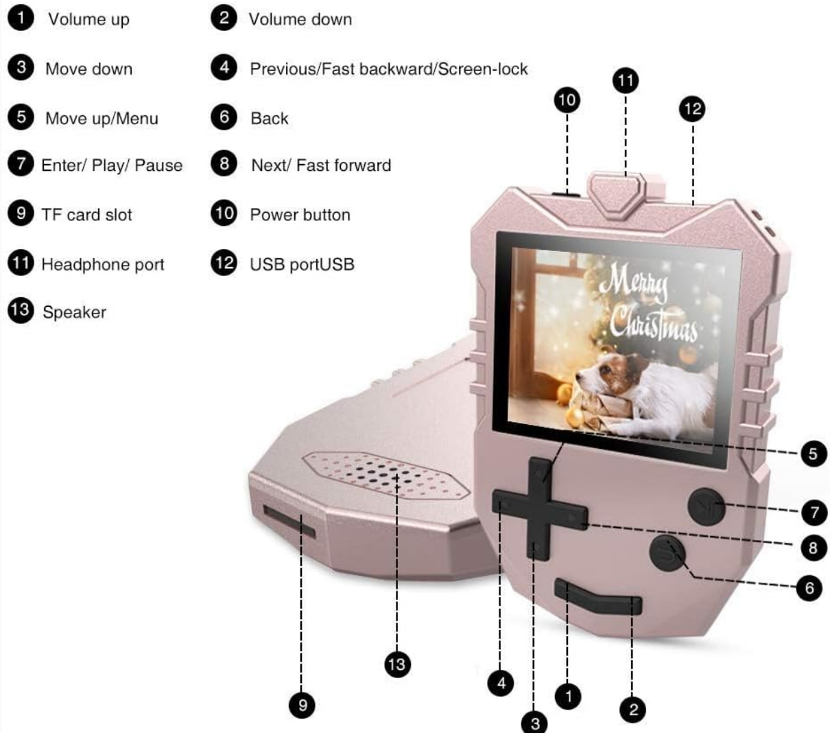
Image: Detailed diagram illustrating the location and function of each button and port on the AGPTEK K1 MP3 Player.
