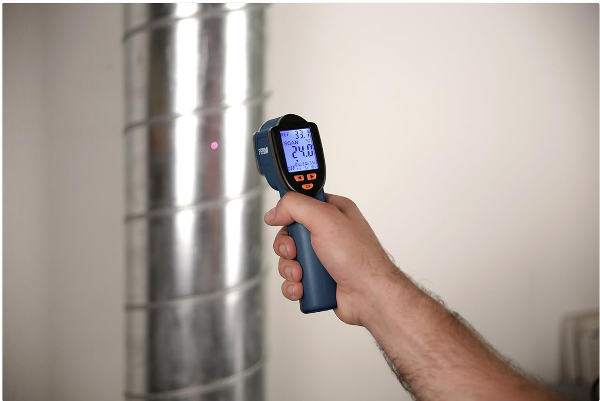
Figure 5.1: User holding the Ferm ITM1001 to measure the temperature of a pipe. The laser dot is visible on the target surface, and the display shows the temperature reading.
