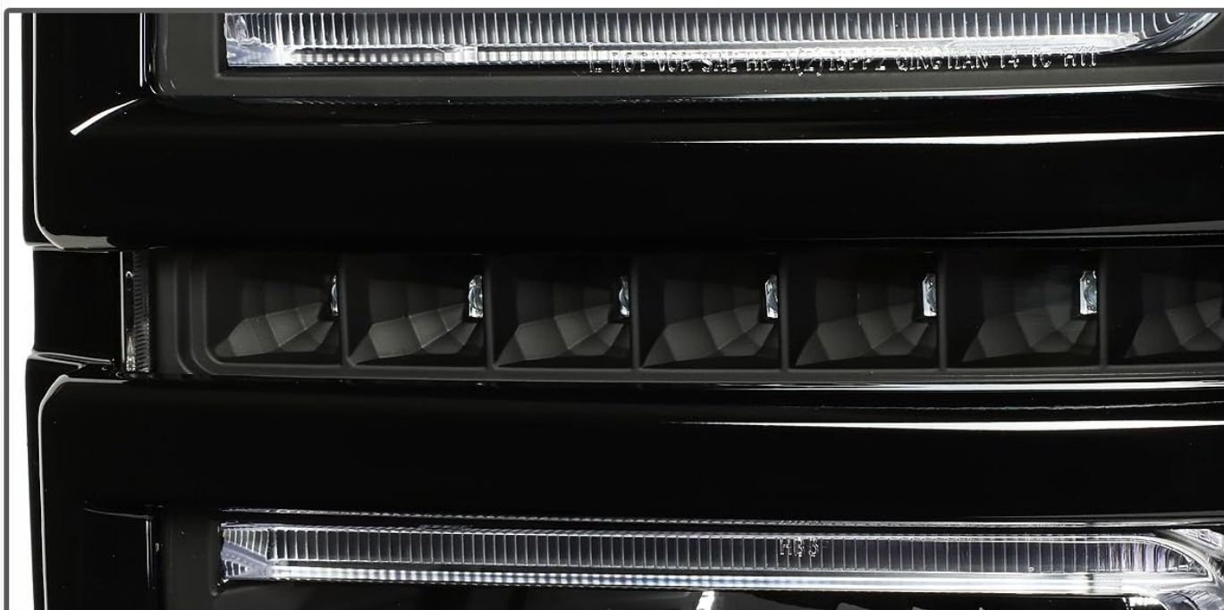
Image 3: Close-up view of the LED strip and reflector details within the DNA MOTORING HL-LB-CS15-BK-AM headlight assembly.
