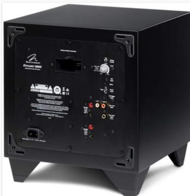
Figure 2: Rear panel showing input and control connections.
