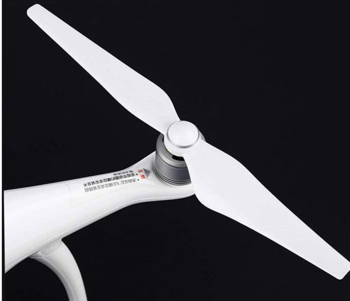
Image: Illustrates the quick-release attachment of a propeller to a DJI Phantom 4 motor.
