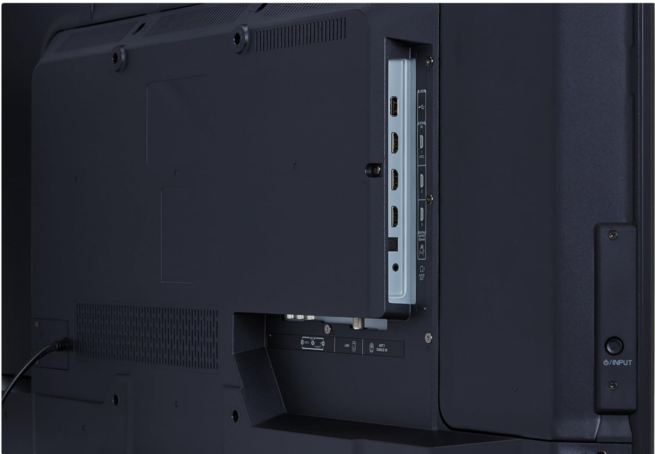
Close-up view of the side-mounted input ports on the Toshiba 43LF621U19, including HDMI and USB connections.
