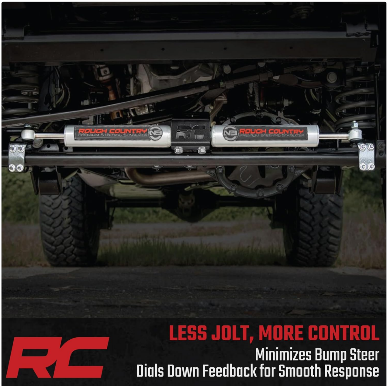
Image 6.1: The stabilizer minimizes bump steer for smoother response.
